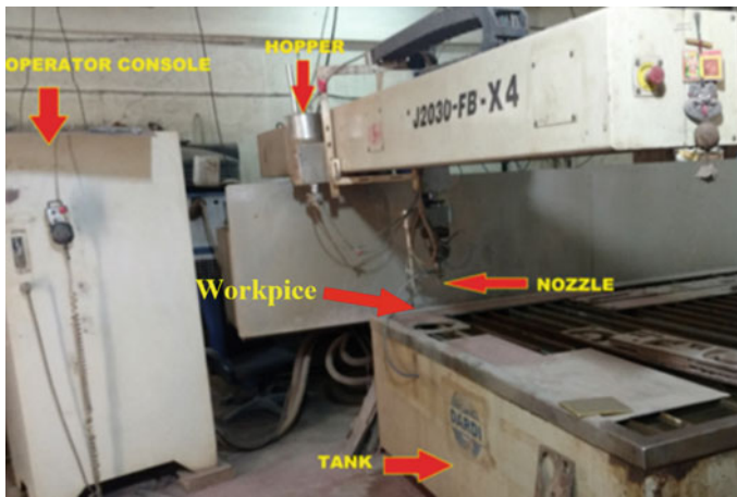
Fig. 4.2 AWJM experimental setup
